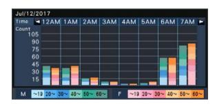
Horizontal axis: When "One hour" is selected for "Scale of the horizontal axis", the statistical graph will be displayed on an hourly basis (up to 24 hours), when "One day" is selected, the statistical graph will be displayed on a weekly basis divided into each day of the week.
