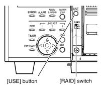
**5** Turn on the power of the recorder by pressing the [POWER] switch while holding down the [USE] button until the buzzer starts sounding.
