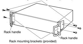
**4** Install the extension unit in the rack by using four rack mounting screws.
