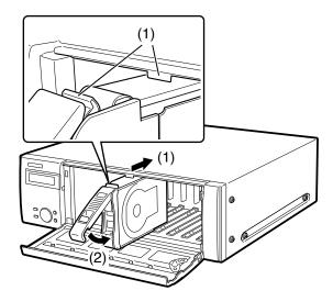
**3** The recognition process of the hard disk drive will start automatically, and then the data recovery will start. When the data recovery starts, the respective HDD access indicator will light orange and red alternately.
