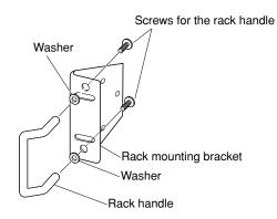
**3** Place the provided rack mounting brackets on both sides of the extension unit and fix them with the rack mounting bracket fixing screw (x6).
